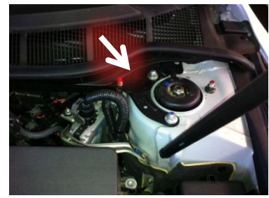
Distress (Green) Light Reset Switch
