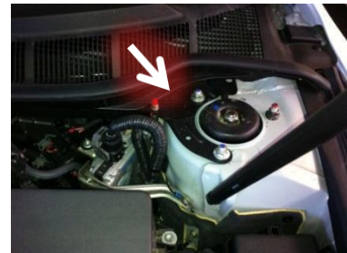
Distress (Green) Light Reset Switch
